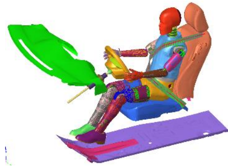
Figure 4: 50%ile dummy model
